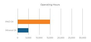
Approximate oil change intervals of gear oils at an operating temp of 80°C
